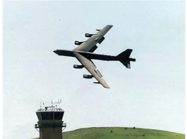
The B-52 on its final steeply banked 360° turn, round the control tower, with flaps and spoilers deployed. From Wikipedia, the free website encyclopaedia.
