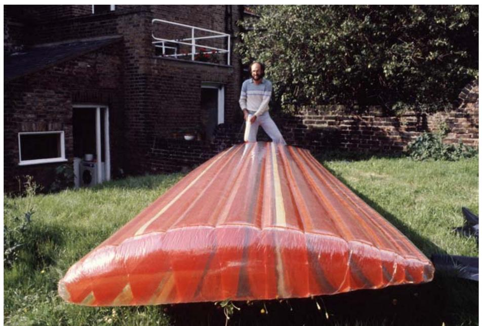
20' span prototype wing for Phoenix
