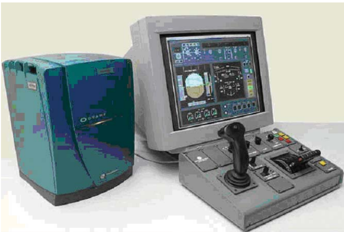
Figure 11. Airbus Desktop Development System.
