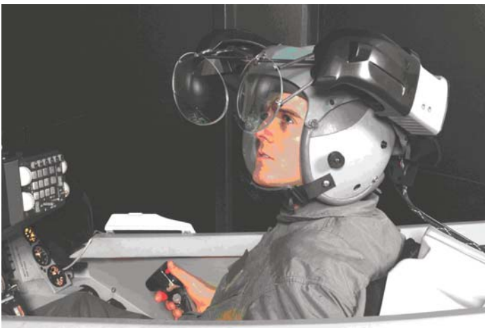
Figure 10. Helmet-mounted visual system.
