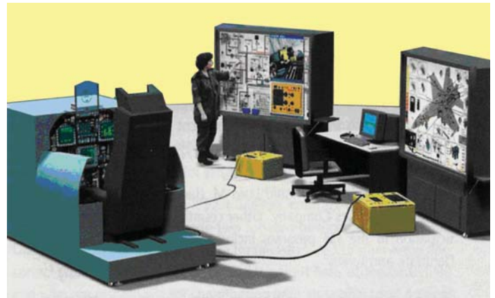
Figure 5. Aircraft maintenance trainer.
