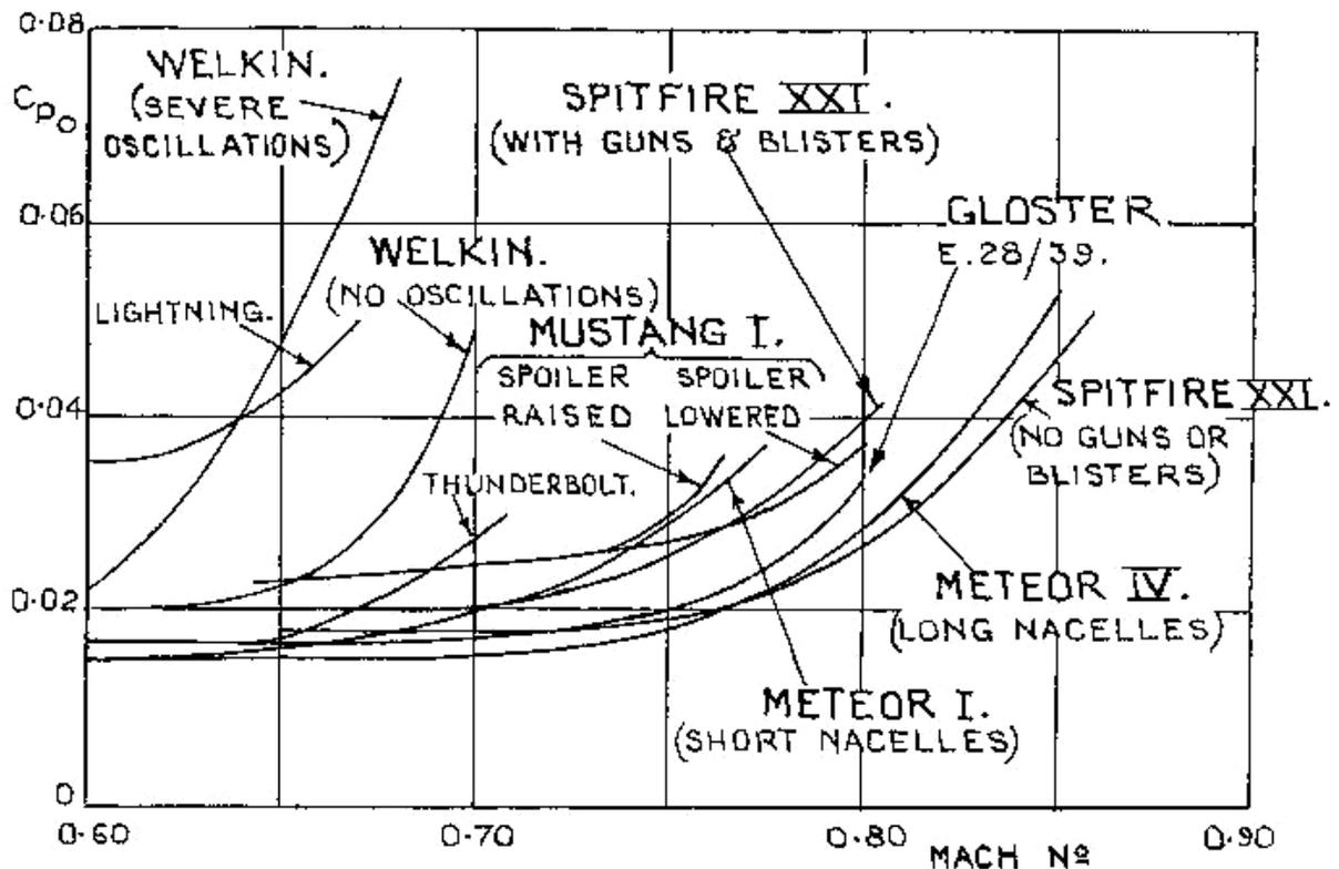
Figure 5 Variation of  $C_{D0}$  with Mach number for various aircraft <sup>(45)</sup>
