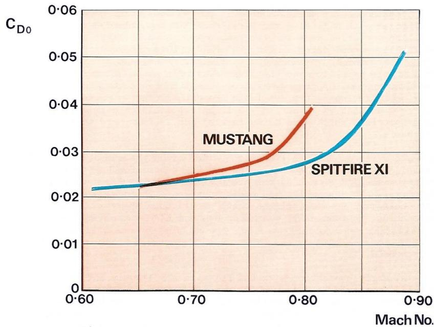
Figure 4 Variation of  $C_{D0}$  with Mach number for the Spitfire PR XI and the P-51 Mustang, from Quill's contribution to Reference 7
