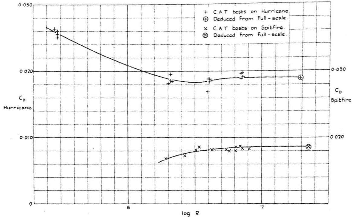
Figure 3 Drag coefficient,  $C_D$ , variations with Reynolds number,  $R$ , for Spitfire & Hurricane models. Collar<sup>(26)</sup>
